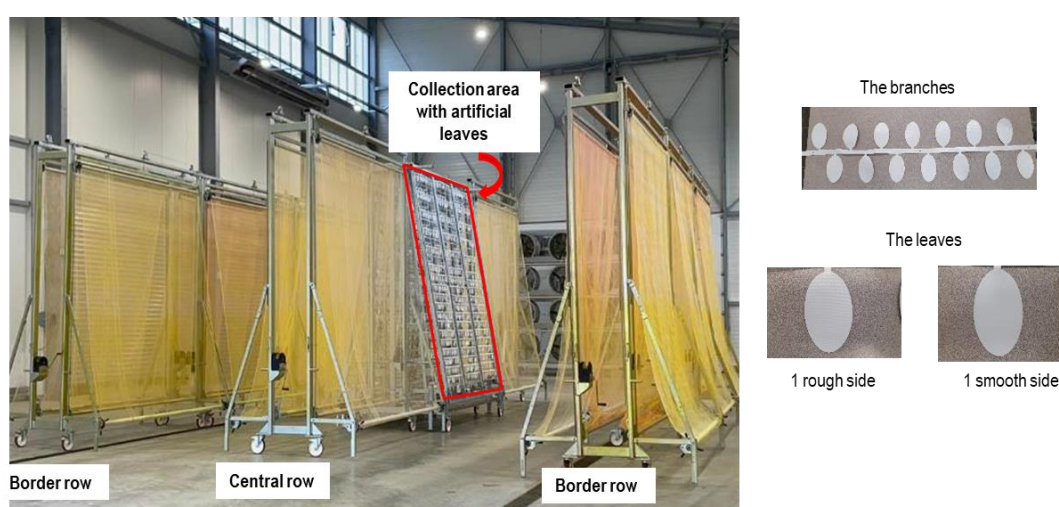
Figure 2: Artificial orchard (a) containing the collect spray deposits system: the branches (b), each with 14 artificial leaves.
